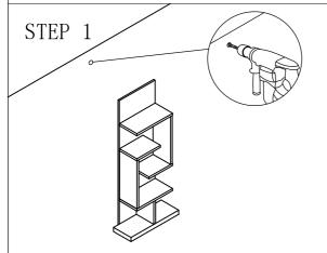
1. Find spot on wall 1'' below top of item. 2. Using a drill bit slightly thinner than anchor ,drill hole into drywall.
