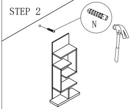
1. Use a light hammer to tap anchor into hole.
