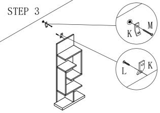
Insert drywall screw into metal bracket and into drywall anchor.
